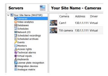
This will open the Cameras tab in the panel to the right of the Servers panel. It is in this panel that you manage cameras/encoders on the specific server that you are dealing with. You need to add the CathexisObserver as you would a camera.
