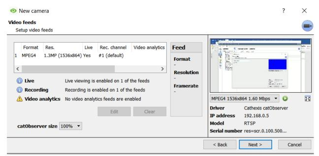
The Video Feeds window follows on from the General Settings Windows. There is a preset stream present, and the live preview pane is still present from the last window. You can edit the settings of the feed by either selecting the feed and then selecting the button; or by simply double-clicking the feed that you want to edit. This will bring up the following window:
